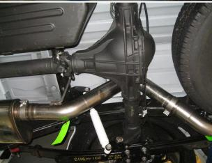
**Step 3.** Install the Muffler to the Inlet Pipe Assembly using the supplied 3.50" clamp. Next install the Over Axle Assembly to the Muffler in the similar fashion using the supplied 3.50" clamp, fitting the welded hangers into the rubber insulators.
