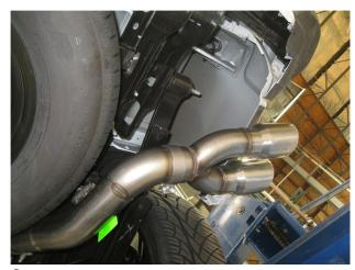
**Step 4.** Finish by installing the Tail Pipe Assembly to the Over Axle Assembly and Tip Assembly to the Over Axle using the supplied 3.50" clamps, fitting the welded hanger into rubber insulator.
