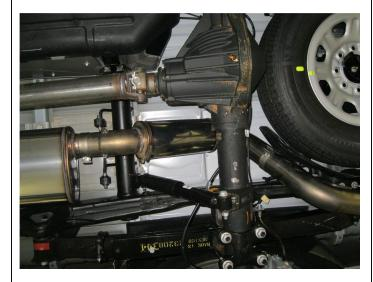
**Step 4.** Next install the over axle Resonator assembly to the Muffler in the similar fashion using the supplied 3.50" clamp, fitting the welded hangers into the rubber insulators.
