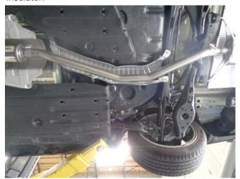
Step 3: Next loosely fasten the Mid Extension Pipe to the Ersonator Assembly using the supplied clamp.
