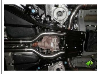
**Step 4.** Next attach the Mid Pipe Assemblies to the Resonator Assembly using the supplied 3.00" clamps and fitting the hangers into the rubber insulators.
