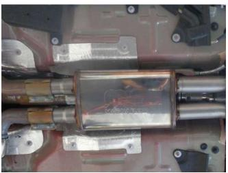
**Step 3.** Begin installation of the new system by loosely attaching the Resonator Assembly to the outlets using the OEM clamps. Leave all clamps loose until final adjustment.
