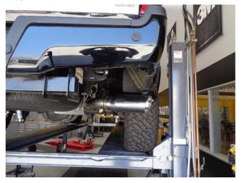
Step 7: Once a final position has been chosen for the new exhaust system, evenly tihgten all clamps from front to rear using the torque specifications on page one of these instructions. Inspect all fasteners after 25-50 miles for operation and re-tighten if necessary.
