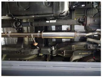
Step 5: If required add the 19.25" Extension Pipe. Loosely attach the Extension Pipe Assembly using the supplied clamp[s]. Engage the welded hanger to the rubber insulator.
