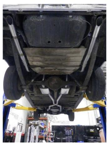
**Step 3.** Once a final position has been chosen for the new exhaust system, evenly tighten all clamps from front to rear using the torque specifications on page one of the instructions. Inspect all fasteners after 25-50 miles of operation and re-tighten if necessary.
