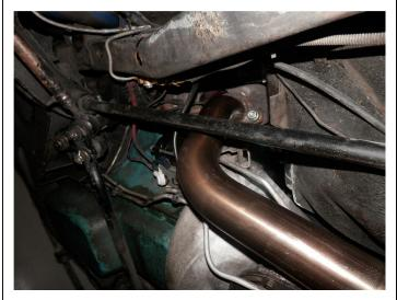
**Step 1.** This install sheet assumes you have already removed the OEM exhaust system. Identify the drivers side and passengers side Manifold Pipes. Drivers side is shown.
