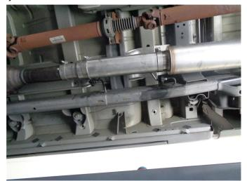
**Step 2.** Install the corresponding Adapter Pipe pertaining to your vehicle and loosely fasten it to the catalytic converter outlet using the supplied clamp. Next, refer to the table below to select the appropriate extension pipes for your vehicles configuration. If applicable loosely attach the Extension Pipe to the Adapter Pipe using the supplied clamp.
