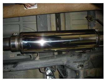
**Step 3.** Loosely attach the Muffler Assembly using the supplied clamps.
