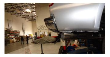
**Step 6.** Once a final position has been chosen for the new exhaust system, evenly tighten all clamps from front to rear using the torque specifications on page one of the instructions. Inspect all fasteners after 25-50 miles of operation and re-tighten if necessary.
