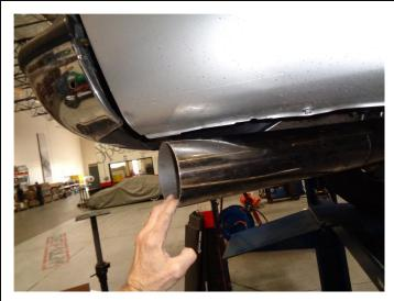
**Step 5.** Install the Tail Pipe Assembly in the same way. The Outlet may be trimmed as desired.
