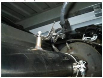
**Step 4.** For year spread 2013 and later with a long bed configuration attach the OEM cable bracket using the OEM bolt. This step is not required on other years or configurations.
