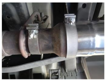
**Step 3.** Begin installation by loosely attaching the Inlet Pipe Assembly to the OEM flange outlet using the OEM hardware (6.7L), or loosely attach the Inlet Adapter to the DPF outlet using the supplied clamp (6.4L). Loosely attach the Extension Pipe, if needed, using the supplied clamp.
