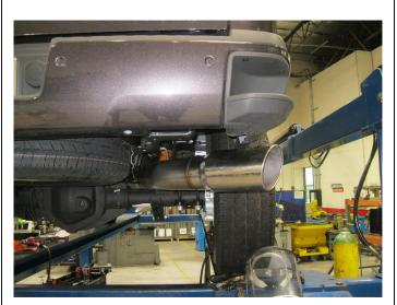
**Step 4.** Once a final position has been chosen for the <u>new exhaust system</u>, evenly tighten all clamps from front to rear using the torque specifications on page one of the instructions. Inspect all fasteners after 25-50 miles of operation and re-tighten if necessary.
