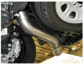
**Step 3.** Next Install the Tail Pipe Assembly in a similar fashion using the supplied 5.00" clamp and by fitting the welded hangers into the rubber insulators.
