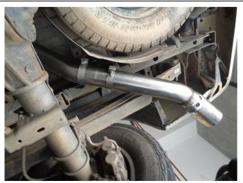
**Step 6.** Next, loosely slip the Hanger Clamp Assembly over the Tail Pipe Assembly and Install using the supplied clamps and by fitting the welded hangers into the rubber insulators.
