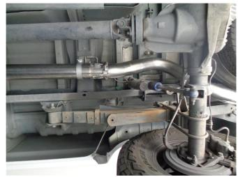
**Step 4.** Loosely install the Over Axle Pipe Assembly using the supplied clamp. Remove the sensor plug for 6.7L application. Loosely slip the Hanger Clamp Assembly over the pipe and locate the welded hangers to the rubber insulators.
