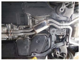
Step 2: Begin installing your new system by loosely attaching the Muffler Assembly by inserting the two inlet pipes into the OEM band clamps at the catalytic converter outlets. Engage both hangers to the rubber insulators.
