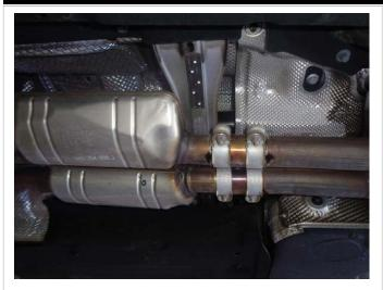
Step 1: To remove the OEM system first loosen both band clamps attaching the exhaust system to the catalytic converter outlet pipes. Working front to rear disengage all welded hangers from the rubber insulators. The OEM exhaust system can now be removed in one piece. Be sure to retain all mounting hardware as it will be needed to install your new MAGNAFLOW system
