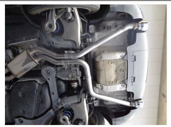
Step 3: Next loosely fasten the Extension Pipe to the passengers side outlet pipe of the Muffler Assembly using the supplied clamp. Then attach both Tail Pipe Assemblies in a similar fashion engaging the welded hangers to the rubber insulators.
