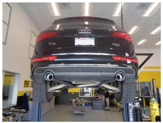
Step 4: Once a final position has been chosen for the <u>new exhaust system</u>, evenly tingten all clamps from front to rear using the torque specifications on page one of these instructions. Inspect all fasteners after 25-50 miles for operation and re-tighten if necessary.
