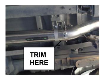
**Step 1.** Locate the rear extension pipe connected to the over the axle pipe as shown in the picture. Measure and trim 17 inches from the rear of the extension pipe. For Chevy applications, trimming is not required since the muffler assembly will replace the rear extension pipe.
