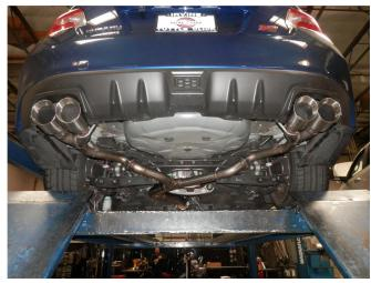
**Step 5.** Next loosely install both Tail Pipes by bolting the inlets flanges to the Y-Pipe Assembly using the OEM hardware. Insert all welded hangers into the OEM rubber insulators.
