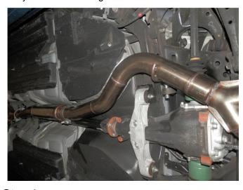
**Step 4.** Next loosely fasten the Y-Pipe Assembly to the Resonator Assembly using the supplied 3.00" clamp. Insert the welded hanger into the OEM rubber insulator.
