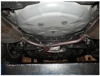
**Step 2.** Next, remove both muffler assemblies by unbolting them from OEM Y-Pipe assembly. Remove all welded hangers from the rubber insulators. The exhaust system may now be removed. Retain all mounting hardware as it will be needed to install your new MAGNAFLOW system.
