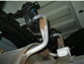
**Step 1.** Begin removal of the OEM system by loosening the clamp at the front of the muffler and disengaging the hangers from the rubber insulators. Working rearward finish removing the system. Do not damage or discard the rubber insulators as they will be re-used to mount the new system.
