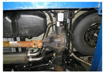
**Step 3.** Next Install the Driver and Passenger side Extension Pipe Assemblies using the supplied 2.50" clamps and fitting the hangers into the rubber insulators.
