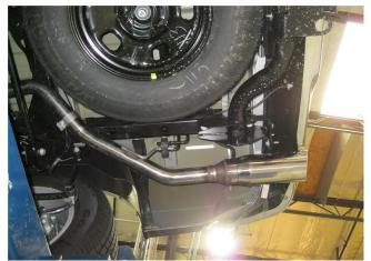
**Step 4.** Complete the installation by fastening the Driver and Passenger side Tailpipe Assemblies to the Extension Pipe Assemblies with the supplied 2.50" clamps and fit the hangers into the insulators.
