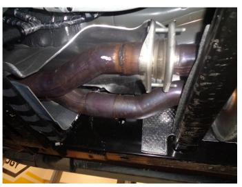
**Step 3.** Finally remove of the OEM inlet muffler assembly by unbolting the inlet at the driver side flange junction and loosening the band clamp on the passenger side inlet pipe. Remove the inlet muffler asembly. You are now ready to install your new MAGNAFLOW exhaust system.
