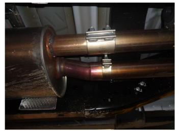
**Step 2.** Next loosen both band clamps attaching the rear muffler subassembly to the inlet muffler assembly. Disengage all welded hangers from the rubber insulators. The muffler subassembly may now be removed.
