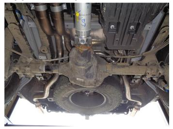
**Step 6.** Loosely attach both Over Axle Pipes to the Muffler Assembly outlet nipples using the supplied clamps.
