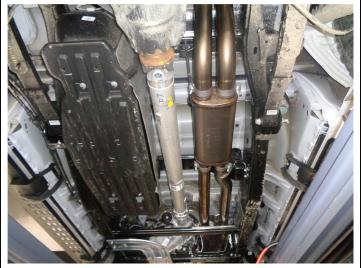
**Step 5.** Install the Muffler Assembly by attaching the the inlet nipples to the outlets of both Inlet Pipe Assemblies. Loosely secure using the supplied clamps. Engage the welded hanger to the rubber insulator.
