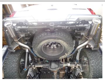
**Step 7.** Lastly loosely attach both Tail Pipe Assemblies to the Over Axles Pipes using the supplied clamps. Engage all welded hangers to the rubber insulators.
