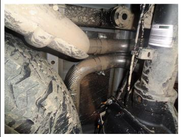
**Step 1.** Begin removal of the OEM exhaust system by loosening the band clamps attaching the tail pipe assemblies to the over axle pipes. Disengage all welded hangers from the rubber insulators and remove both tail pipes. Retain all mounting hardware as it will be used to install your new system.
