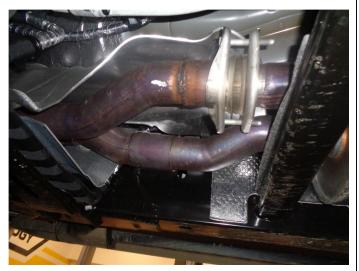
**Step 3.** Finally remove the OEM inlet muffler assembly by unbolting the inlet at the driver side flange junction and loosening the band clamp on the passenger side inlet pipe. Remove the inlet muffler asembly. You are now ready to install your new MAGNAFLOW exhaust system.
