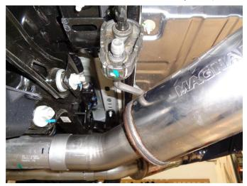
**Step 3.** Begin installation of the new system by sliding the D/S Muffler Assembly inlet onto the cut outlet of the OEM exhaust and loosely fasten with the supplied 2.75" clamp. Fit the hangers into the rubber insulators.
