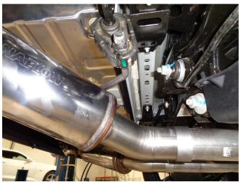
**Step 4.** Install the P/S Muffler Assembly in the same manner. Leave all clamps loose for final adjustment of the system.
