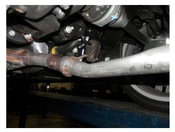
**Step 2.** Cut the passengers side tail pipe in a similar fashion measuring 15" rearward of the welded hanger as show. Again, deburr cut edge. You are now ready to install your new MAGNAFLOW system.
