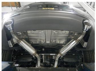
**Step 3.** Begin installation by loosely attaching both drivers side and passengers side Muffler Assemlies to the outlet of the cut pipes using the supplied clamps and fitting the hanger into the rubber insulator. Leave all clamps loose until final adjustment
