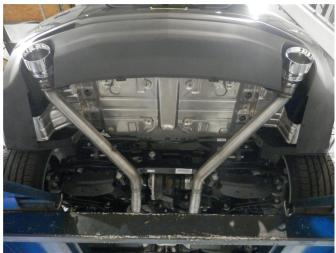
**Step 3.** Begin installation by loosely attaching both drivers side and passengers side Tail Pipe Assemlies to the outlet of the cut pipes using the supplied clamps and fitting the hanger into the rubber insulator. Leave all clamps loose until final adjustment
