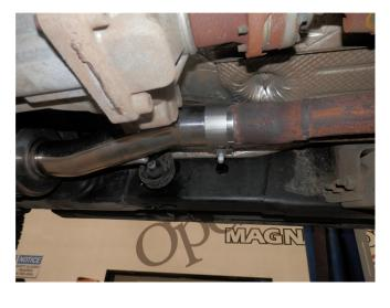
**Step 3.** Begin installation of your new MAGNAFLOW system by attaching the Resonator Assembly to the catalytic converter outlet using the OEM band clamp. Align the locating peg with the notch in the inlet pipe. Engage the welded hanger to the rubbe insulators. Keep all fasteners and clamps loose until final adjustment.
