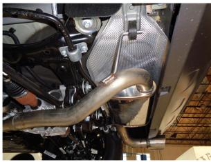
**Step 4.** Mount the Muffler Assembly to the Mid Pipe with the supplied 2.50" clamp and locate both welded hangers into the OEM rubber insulators.
