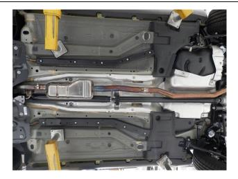
**Step 1.** To remove the OEM exhaust loosen the factory clamps in front of and behind the factory resonator assembly. Disengage all welded hangers from the rubber insulators. Retain rubber insulators as they will be needed to install your new MAGNAFLOW system. The OEM system can now be removed.
