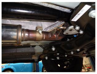
**Step 2.** Begin installation of your new MAGNAFLOW system by slipping the Resonator Assembly inlet end over the Catalytic Converter outlet locating the alignment pin into the coresponding slot on the Resonator inlet. Loosely secure using the supplied 2.25" clamp. Leave all clamps loose during initial installation.
