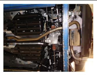
**Step 3.** Next, attach the Mid Pipe to the Resonator Assembly outlet using the supplied 2.50" clamp.
