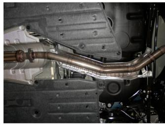
**Step 4.** Next attach the Y-Pipe Assembly to the Inlet Resonator Assembly by coupling the flanges using the supplied gasket and hardware.
