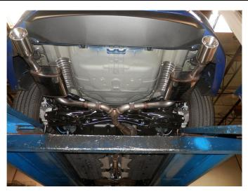
**Step 5.** Loosely attach both driver and passenger side Muffler Assembly flanges to the Y-Pipe Assembly. Secure with the supplied gaskets and hardware. Engage welded hangers to rubber isolators.
