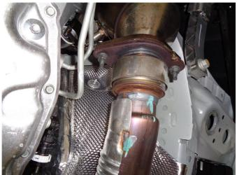
**Step 1.** To remove the OEM exhaust you will need to unbolt and remove the cross brace shown. Now you can unbolt the OEM exhaust from the catalytic converter flange junction. Disengage all welded hangers from the rubber insulators. Retain rubber insulators as they will be needed to <u>install your new MAGNAFLOW system</u>. The OEM system can now be removed.
