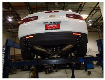
**Step 5.** Once a final position has been chosen for the <u>new exhaust system</u>, evenly tighten all clamps from front to rear using the torque specifications on page one of the instructions. Inspect all fasteners after 25-50 miles of operation and re-tighten if necessary.
