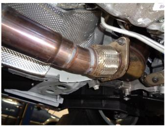
**Step 2.** Begin installation of your new MAGNAFLOW system by loosely bolting the Inlet Pipe Assembly to the catalytic converter outlet flange using the OE fasteners.
