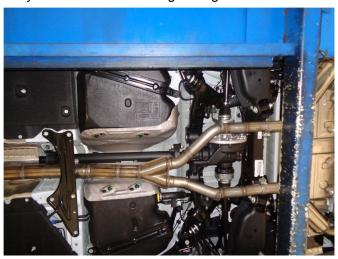
**Step 3.** Next, loosely install the Y-Pipe Assembly using the supplied 3.00" clamps. Locate the welded hangers to the rubber insulators.
