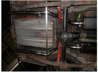
**Step 5.** Next, loosely attach the desired Tail Pipe Options using the suppled clamps.
