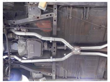
**Step 1.** Begin installation of you new exhaust system by loosely installing the two Inlet Pipes to the installed Magnaflow Manifold Front Pipes (sold separately) using the supplied clamps. These pipes may need to be trimmed to assure correct fitment.
