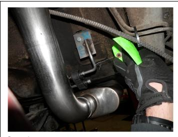
**Step 3.** Use suppled Hanger Brackets to mount both Muffler Assemblies. Secure using the supplied hardware.
