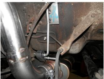
**Step 4.** The extra Hanger Bracket supplied is for vehicles that came stock with one tail pipe. This bracket is to be located to the E-Brake cable bracket. Loosely secure with the supplied hardware.
