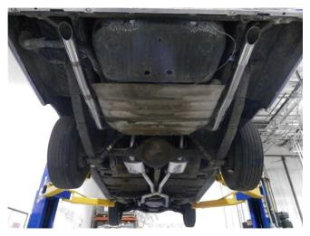
**Step 8.** Once a final position has been chosen for the new exhaust system, evenly tighten all clamps from front to rear using the torque specifications on page one of the instructions. Inspect all fasteners after 25-50 miles of operation and re-tighten if necessary.
