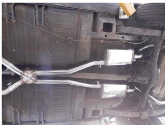
**Step 2.** Loosely attach the X-Pipe Assembly to the Inlet Pipes and then the Muffler Assembles to the X-Pipe Assembly using the suppled clamps.
