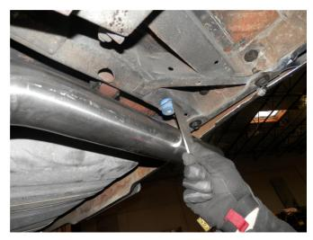
**Step 6.** Secure the Tail Pipes with the supplied Tip Hanger Brackets and Snap Grommets. Try to position each bracket to locate an existing hole in the vehicles sub frame to avoid drilling. Once the desired position has been found mark its location. Trim the bracket as necessary and bolt the bracket with the Snap Grommet to the sub frame using the supplied hardware. Weld the bracket to the Tail Pipe once you have the pipe in position.
