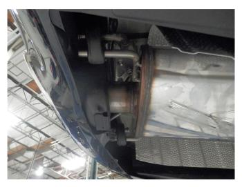
**Step 3.** Begin installation of your new MAGNAFLOW system by attaching the Inlet Pipe Assembly to the catalytic converter outlet using the OEM fasteners and insulator. Keep all fasteners and clamps loose until final adjustment.
