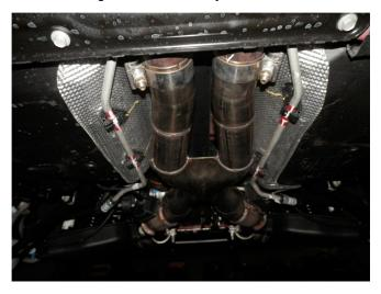
**Step 4.** Begin installation of the new system by sliding the X-Pipe Assembly inlets onto the cut outlets of the OEM exhaust and loosely fasten with the supplied 2.75" clamps. (at this time slide the loose end of the cut heatshield under the clamps before tightening). Fit hangers into rubber insulators.
