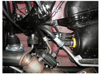
**Step 6.** To re-connect the wiring harness plugs to the Valve motors you may need to cut their plastic anchors. After having done this attach the plugs to the motors and re-anchor the wires with a supplied Zip Tie.
