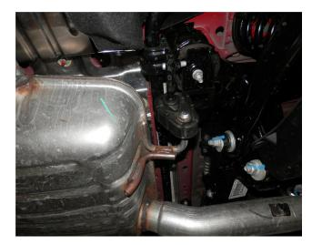
**Step 3.** Working front to rear disengage all welded hangers from the rubber insulators and remove the system. (Retain the insulators as they will be needed to mount the new MAGNAFLOW system.) Once the OEM system is on the ground transfer all the valve motors over to the new Magnaflow exhaust system.
