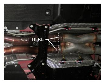
**Step 1.** It is necessary to cut the factory exhaust system to install the new Magnaflow unit. To do this cut the band clamps holding the heat shield to the pipes in front of the X. Move the heatshield out of the way and cut 1/2" in front of the welds on the factory X-Pipe. Deburr the cut pipes to facilitate installation of the new system.
