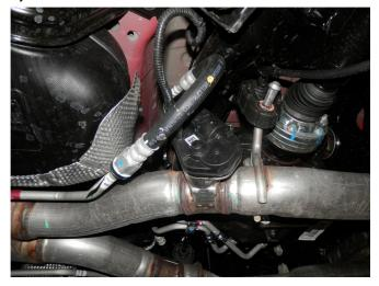
**Step 2.** Next you will need to unplug the electrical connection on the Exhaust Valve Control Motors (Qty 4) located on the OEM exhaust assembly.
