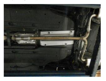
**Step 3.** Next Install the Y-Pipe Assembly to the Inlet Pipe Assembly using the supplied 2.50" clamp. Insert hanger into rubber insulator.
