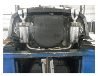
**Step 4.** Finish by Installing the Muffler Assemblies to the outlets of the Resonator Assembly using the supplied 2.50" clamps. Insert hangers into rubber insulators.
