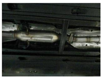
**Step 2.** This Magnaflow exhaust system will fit both a 2.0LTurbo and a NA 2.4L Optima depending on which Inlet pipe Assembly is used (both are supplied). The 2.0L Turbo Inlet Pipe has the slotted flange. Begin installation of the new system by fastening the correct Inlet Assembly to the resonator outlet using the OEM fasteners (Leave all clamps and fasteners loose for final adjustment of the complete system.)
