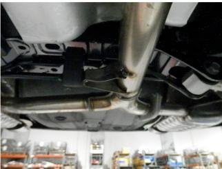
**Step 1.** To extract the OEM exhaust system begin by un-fastening the flange located behind the resonator and the second flange located in front of the Driver side muffler assembly. Next, working rearward, disengage all welded hangers from the rubber insulators. Do not damage or discard the rubber insulators or fasteners as they will be re-used to mount the new system. You can now remove the exhaust from the vehicle.
