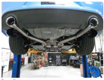
**Step 5.** Loosely install both Tail Pipe Assemblies using the supplied clamps. Attach the welded hangers to the rubber insulators.
