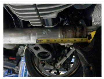
**Step 1.** Begin removal of the OEM system by cutting both sides of the systems exhaust pipes. For the drivers side cut 4" rearward of the outlet weld on the exhaust control valve as shown in the attached picture.
