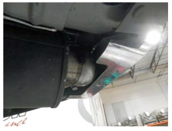
**Step 3.** Next, loosen the band clamps attaching the rear muffers to the OEM tips. Disengage all welded hangers from the rubber insulators. You may now remove the rear exhaust system. Do not discard or damage the rubber insulators as they will be used to install the new exhaust system.
