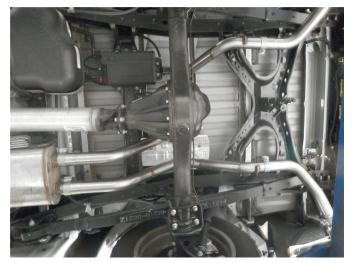
**Step 2.** Begin installing of the new system by attaching both of the Inlet Pipe Assemblies to the outlets of the OEM system using the OEM hardware. Next attach the Mufler Assembly to the inlet pipes with supplied clamps and insert the hangers into the rubber insulators. Keep all clamps loose for final adustment of the system.
