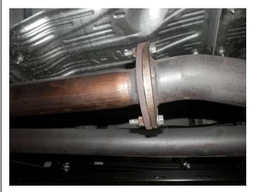
**Step 1.** To begin the removal of the OEM system you will need to remove the spare wheel. Next unbolt both inlet flanges at the OEM inlet ipie assembly. Working rearward (with the exhaust supported) extract the hangers from the rubber insulators and remove the OEM exhaust. Do not discard or damage the rubber insulators as they will be used to install the new exhaust system.
