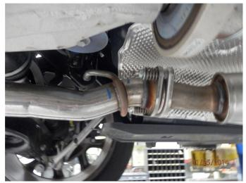
**Step 1.** Begin removal of the OEM system by cutting both side of the systems exhaust pipes. For the drivers side cut 11" rearward of the welded hanger behind the flange junction as shown in the attached picture.
