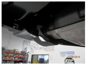
**Step 5.** To install the Quad Tip option supplied you will first need to remove the OEM tips from the vehicles valence. Remove the four bolts attaching each tip with a 10mm socket.
