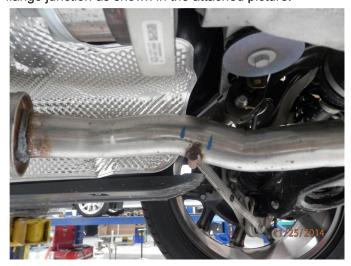
**Step 2.** For the passengers side cut 11" rearward of the welded hanger behind the muffler as shown in the attached picture. Next un-clip the ground strap from the passenger side muffler hanger. With the exhaust supported extract the hangers from the rubber insulators and remove the OEM muffler assemblies. De-burr and smooth the cut pipes to prepare them for the new exhaust. Do not discard or damage the rubber insulators as they will be used to install the new exhaust system.
