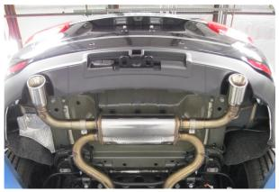
**Step 6.** Next install the Tailpipe Assemblies using the supplied 2.50" Clamps and fit the hangers into the rubber insulators.
