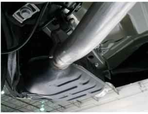
**Step 2.** Working rearward disengage the remaining hangers from the rubber insulators while supposrting the system. Once all hangers are free you can remove the OEM system.
