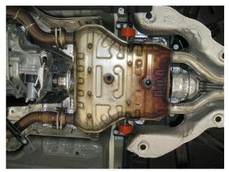
**Step 1.** Begin removal of the OEM exhaust system by unfastening the spring loaded flanges in front of the OEM resonator and disengaging the hangers from the rubber insulators. Retain all hardware and rubber insulators as they will be re-used to install the new Magnaflow system.
