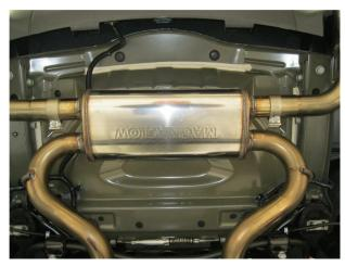
**Step 5.** Next install the Muffler Assembly to the X-Pipe Assembly using the supplied 2.50" Clamps and fit the hangers into the rubber insulators.
