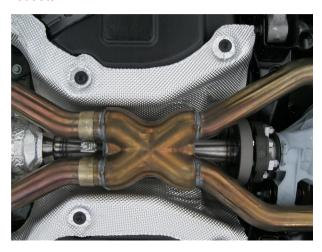
**Step 4.** Attach the X-Pipe Assembly to the Resonator Assemblies using the supplied 2.50" clamps.
