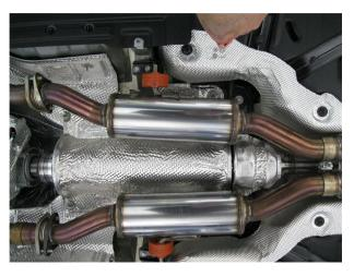
**Step 3.** Begin installation of the new Magnaflow system by using the supplied M10 bolts and OEM nuts to attach the Driver and Passenger Side Resonator Assemblies to the catalytic converter outlets.
