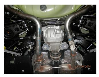
**Step 2.** Begin installation of your new system by slipping each Inlet Pipe Assembly over the cut OEM outlet pipes. Loosely secure using the supplied 2.25" clamps. Locate the welded hangers to the rubber insulators. Remember to re-attach the ground strap to the hanger
