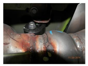
**Step 4.** To install the OEM tips they must first be removed from the stock exhaust system. You will need to loosen the tip clamps and break the weld holding them to the mufflers, both sides.
