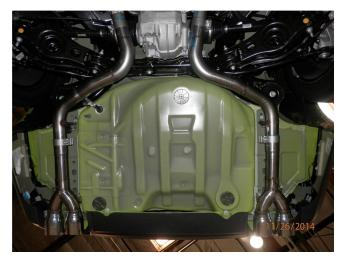
**Step 3.** At this point you have two options for tips. Magnaflow supplies a Quad tip setup that can be clamped to the Inlet Pipes and held in place with hangers and the installation is complete.
