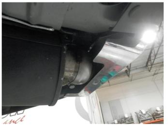
**Step 3.** Next, loosen the band clamps attaching the rear muffers to the OEM tips. You may now remove the rear exhaust system. Disengage all welded hangers from the rubber insulators. Once the two mufflers are removed from the vehicle detach the OEM tip clamps by gently breaking the welds securing them Do not discard or damage the clamps or rubber insulators as they will be used to install the new exhaust system.
