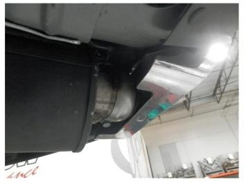
**Step 6.** To install the Quad Tip option supplied you will first need to remove the OEM tips from the vehicles valence. Remove the four bolts attaching each tip.
