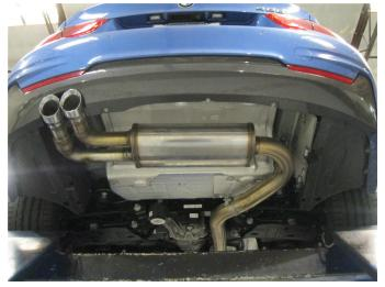
**Step 4.** Install the Muffler Assembly using the same procedure as the Inlet Resonator Assembly with the supplied 3.00" clamp. Engage the welded hangers to the rubber insulators using the OEM hardware. Reattach the connector plug for the exhaust control valve motor.
