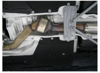
**Step 2.** You will need to cut the OEM exhaust pipe at the inlet weld of the stock resonator. Disengage all welded hangers from the OEM rubber insulators. Do not discard the OEM fasteners or damge the rubber insulators as the will be needed to mount your new MAGNAFLOW system. Once the OEM system has been removed you can unbolt the exhaust control valve motor. Be sure to retain the indexing spring shown in the diagram for Step 1.
