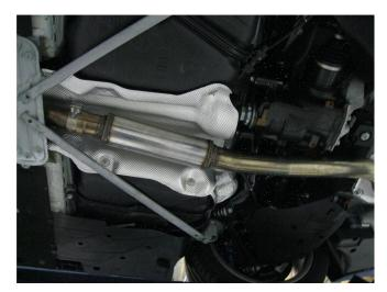
**Step 3.** Loosely Install the Inlet Resonator Assembly using the supplied 3.25" clamp. At this point the OEM exhaust control valve can be bolted to the new Muffler Assembly. Align the keyways in the stock motor and insert the new valve assembly using the OEM indexing spring. **\*\*NOTE: Do NOT loosen or undo the V-Band Clamps, they are designed for one time use only. Once the clamp is tightened it can not be reused.**
