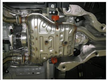
**Step 1.** Begin removing the OEM exhaust system by unbolting the two flanges in front of the main muffler. Working front to rear remove all welded hangers from the rubber insulators. The OEM exhaust system can now be removed in one piece. Retain all mounting hardware and rubber insulators as they will be needing to mount your new MAGNAFLOW system.
