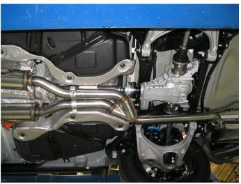
**Step 3.** Loosely install the Y-Pipe Assembly to the two Resonator Assemblies using two of the suppled 2.50" clamps.
