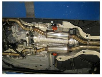
**Step 2.** Begin installing your new system by first loosely attaching both Resonator Assemblies to the vehicle outlet flanges using the four supplied M10 bolts.
