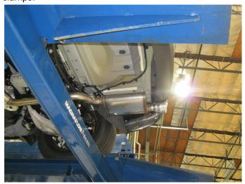
**Step 4.** Install the Muffler Tail Pipe Assembly in a similar fashion using the remaining 2.50" clamp. Locate all welded hangers to the rubber insulators.
