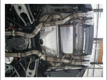
**Step 5.** Install the Muffler Assembly using the same procedure for the V-Band Clamp. Engage the hanger bracket using the OEM hardware.
