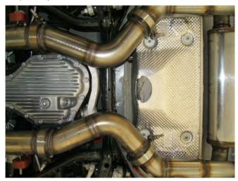
**Step 4.** Loosely Install the D/S and P/S Mid Pipe Assemblies with the supplied V-Band Clamps. \*\*NOTE: Take care when using the V-Band Clamps, they are designed for one time use only. Once the clamp is tightened it can not be reused.
