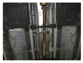
**Step 2.** Begin installation of your new MAGNAFLOW system by attaching the Resonator Assembly to the catalytic converter outlet using the OEM fasteners and insulator. Keep all fasteners and clamps loose until final adjustment.
