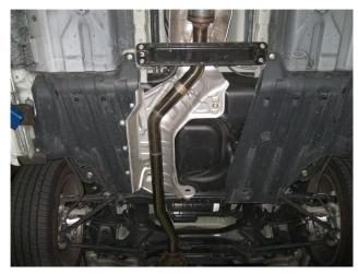
**Step 3.** Next use the supplied 2.25" clamp to attach the Y-Pipe Assembly to the Resonator Assembly and insert the hanger to rubber insulator.
