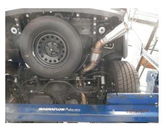
**Step 3.** Complete the initial installation by attaching the Extension Pipe Assembly (containing the exhaust valve) to the Muffler and the Resonator/Tailpipe Assembly the Extension Pipe using the suplied 3.50" clamps.
