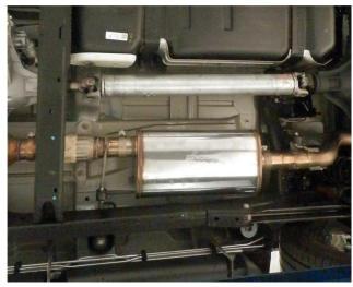
**Step 2.** Begin installation of the new system by attaching Inlet Pipe Assembly at the ball flare using the OEM clamp and fitting the hanger into the rubber insulator. Next attach the muffler to the inlet pipe using a supplied 3.50" clamp. Leave all clamps loose for final adjustment of the complete system.
