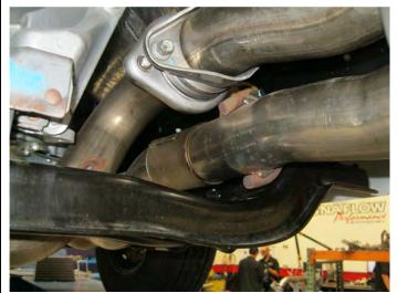
**Step 1.** To remove the OEM exhaust system, unbolt the flange and clamp attaching the systems inlet pipes to the catalytic converter outlet pipes. Disengage all welded hangers from the OEM rubber insulators. Do not discard the OEM fasteners or damage the rubber insulators as they will be needed to mount your new MAGNAFLOW system.
