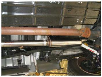
**Step 4.** Install both the Muffler Assembly and Tail Pipe Assembly using the supplied 3.50" clamps. Locate the welded hangers to the OEM rubber insulators.
