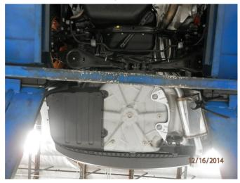
**Step 4.** Next attach the Muffler Assemby to the Resonator Assembly using the supplied 3.00" clamp and by fitting the hangers into the rubber insulators.
