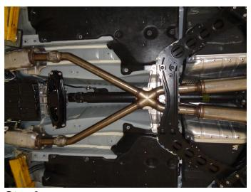
**Step 3.** Install the new X-Pipe Assembly by loosely bolting it to the catalytic converter outlets using the OEM gaskets and fasteners.
