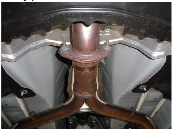
**Step 2.** Unbot the flanges coupling the inlet pipe assembly to the resonator assembly. You may also unbolt the muffler assembly to ease the system removal process. Working front to rear disengage all welded hangers from the rubber insulators. Retain all mounting hardware as it will be needed to install your <a href="new MAGNAFLOW system">new MAGNAFLOW system</a>.
