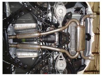
**Step 5.** Install the Muffler Assembly by loosely attaching the inlets to the Resonator Assembly outlets using the supplied clamps. Locate the welded hangers to the rubber insulators.
