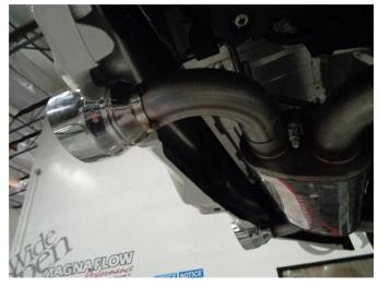
**Step 6.** Install both Tail Pipe Assemblies to the Muffler Assembly. Loosely secure using the supplied clamps.
