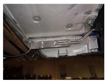
**Step 3.** Next, loosely install the Hanger Bracket to the bracket on the Muffler Assembly using the supplied hardware. Locate the hanger to the rubber insulator.
