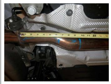
**Step 1.** Begin removal of the OEM muffler by cutting the exhaust pipe 10" forward of the welded hanger in front of the OE muffler as shown. Disengage the welded hanger from the rubber insulator and remove the muffler assembly. Deburr the cut pipe. Retain all OEM hardware as it will be needed to install your new MAGNAFLOW system.
