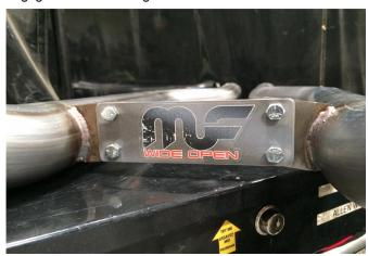
**Step.4** Finally install the MF logo Support Bracket to the welded brackets located on the Mid Pipe Assemblies using the supplied hardware.
