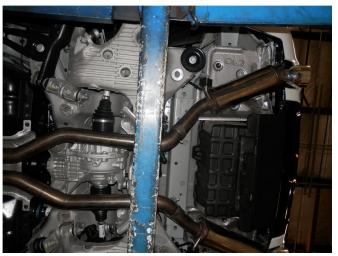
**Step 3.** Next loosely Install the two Mid Pipe Assemblies and the muffler assemblies using the supplied 2.50" clamps. Engage the welded hangers to the rubber insulators.
