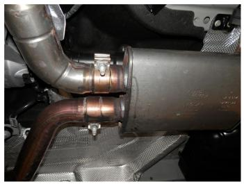
**Step 1.** Begin removal of the OEM system by unclamping the OEM muffler from the catalytic converter outlet pipes. You can then disengage the welded hangers from the rubber insulators, working rearward finish removing the system. Do not damage or discard the rubber insulators as they will be re-used to mount the new system.
