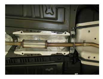
**Step 2.** Begin installation of the new system by fastening the Resonator Assembly inlet to the catalytic converter using the supplied 2.25" clamp (Leave all clamps and fasteners loose for final adjustment of the complete system).
