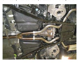
**Step 3.** Next attach the Extension Pipe Assemblies to the Y-Pipe using the supplied 2.50" clamps and fitting the hangers into the rubber insualtors.
