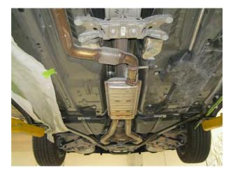
**Step 1.** (Notice: This exhaust system fits on both convertible and coupe Mustangs. To install the system on a convertible you must first remove all underbody bracing.) Begin removing the exhaust system by loosening the clamp located in front of the resonator. Next, working front to rear extract the hangers from the rubber insulators and remove the OEM system. Retain insulators and clamps as they will be used to install the new system.
