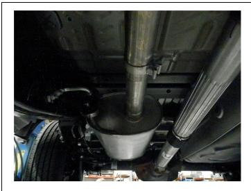
**Step 1.** To remove the OEM exhaust system, loosen the clamp attaching the systems inlet pipe to the resonator outlet pipe. Disengage all welded hangers from the OEM rubber insulators. Do not discard the OEM clamp or damage the rubber insulators as they will be needed to mount your new MAGNAFLOW system.
