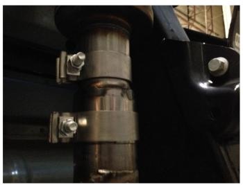
**Step 3.** Install the Extension Pipe between the Inlet Pipe Assembly and the Muffler Assembly using the supplied 3.00" and 2.50" clamps. Engage the welded hanger to the rubber insulator.
