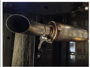
**Step 4.** Install both the Turn Down Tip with the supplied 2.50" clamp.
