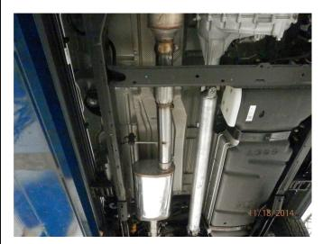
**Step 2.** Begin installation of the new system by attaching Inlet Pipe Assembly at the ball flare using the OEM clamp and fitting the hanger into the rubber insulator. Next attach the muffler to the inlet pipe using a supplied 3.50" clamp. Leave all clamps loose for final adjustment of the complete system.
